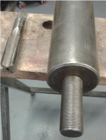
**Plate 2 - Mounting bar showing the threaded stud for attaching the Planer**
